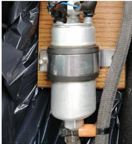
**FIGURA 8:** BOMBA DE COMBUSTIBLE EXTERNA
