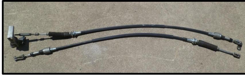
Figura 3.27 Cables de mando push-pull
