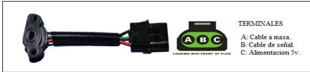
Figura.2.6 Terminales Sensor TPS
