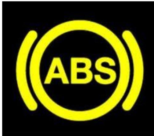
Figura 1.22 Luz testigo ABS
