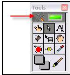
*Figure 22.14: Automatic Tool Selection from the Tools Palette*
