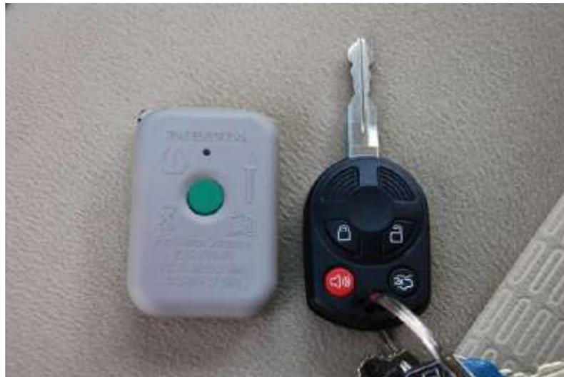
Figura 3.6: Herramienta fordtrigger.
