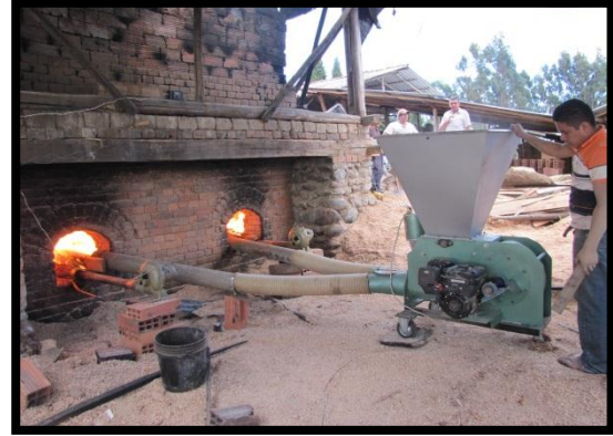
Photo 12: Use of a dispenser to burn excess sawdust
