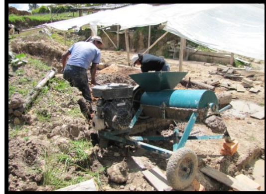
Photo 4: Use of the mixing machine. Swisscontact, 2011
