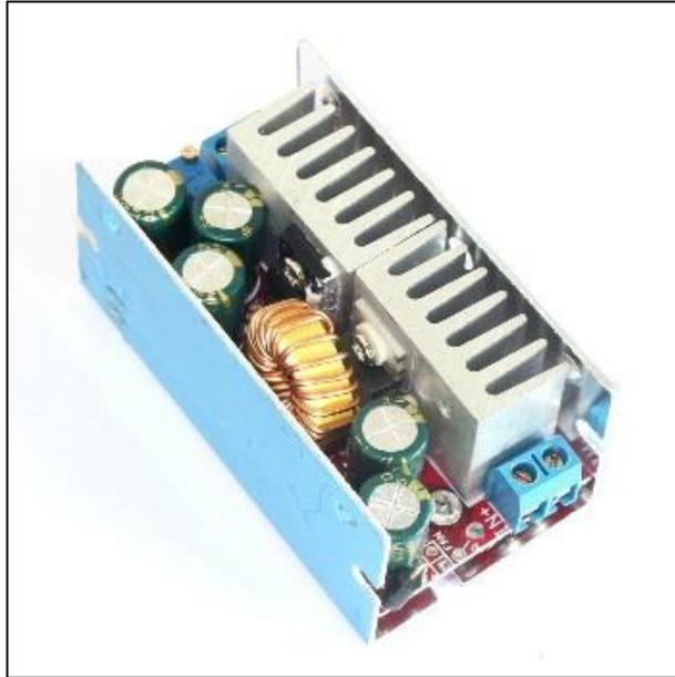
Figura 59 Step Down converter
