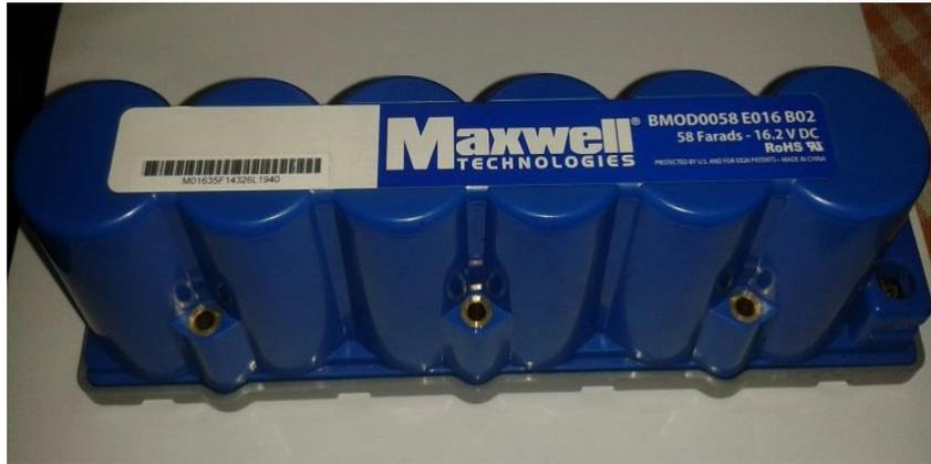
Figura 2. 7 Modulo SC Maxwell 58farads/16.2 VDC
