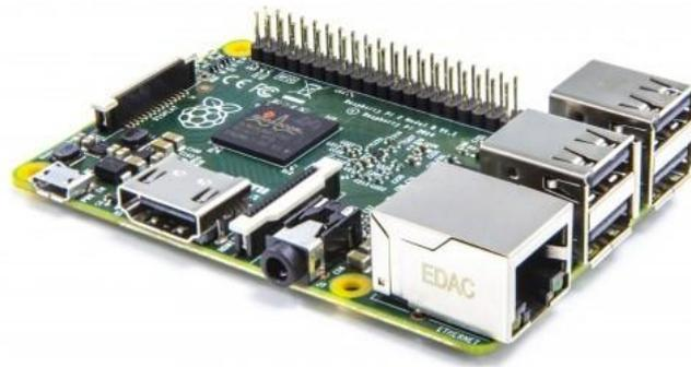
Figura 2.4: Raspberry Pi 2 model B.
