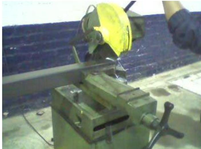
Figura 2-73: Cortes a  $90^{\circ}$
