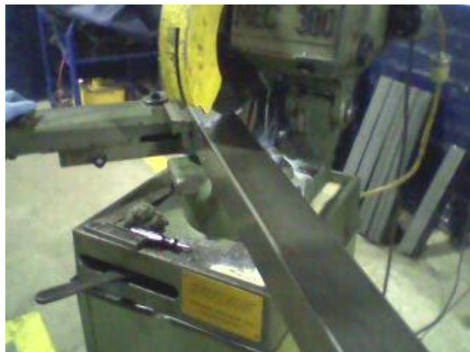
Figura 2-74: Cortes a  $45^{\circ}$
