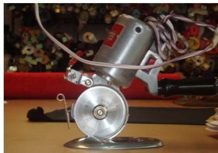
**Figura # 15: Cortadora Vertical**
