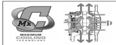
Draws air from drive end and terminal end over electronics and internal components and out frame air vents for cooler internal alternator temperature. These design enhancements also make MxC alternators exceptionally resistant to debris and contamination.
