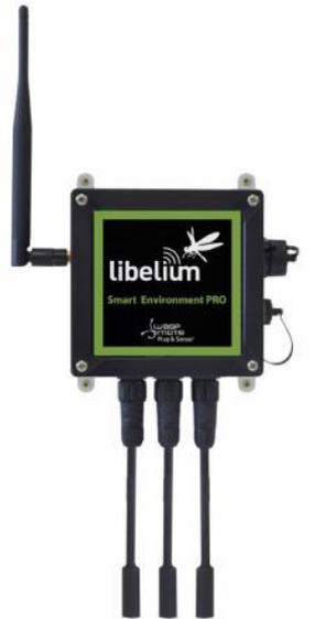
Figura 3.14: Nodo Smart Environment PRO Waspnote Plug & Sense.
