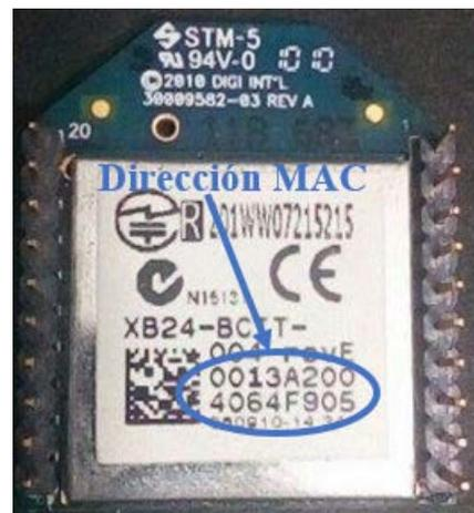
Figura 2.17: Xbee B.
