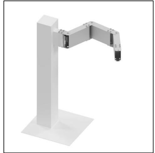
Fig. 7 Robot redundante planar 3R.
