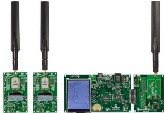
Figura 6. LoRa Technology Evaluation Kit 915MHz-RN2903 [21].
