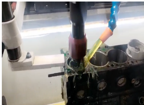
Figura 22 Pistones a 76.0mm
