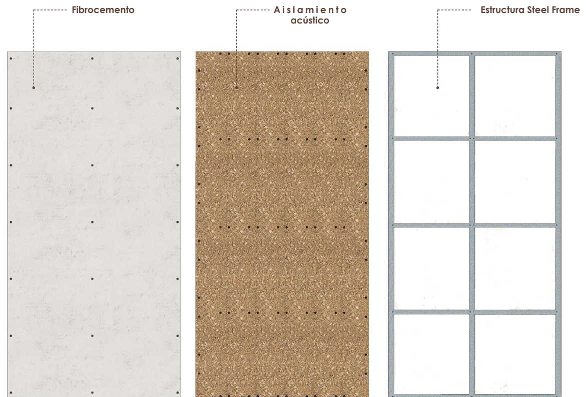
Figura 99: Panel de steel frame
