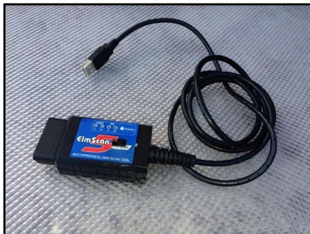
*Figura 5.2. Transceiver OBD2 ELMSCAN5*
