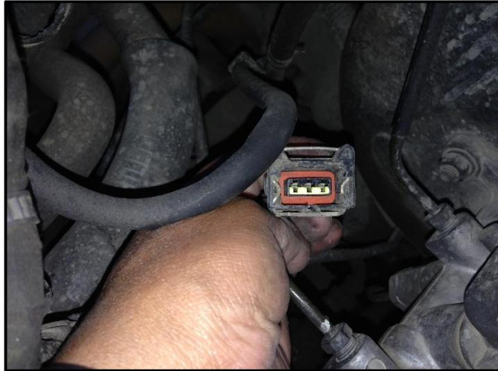
*Figura 5.10. Conector sensor VSS*
