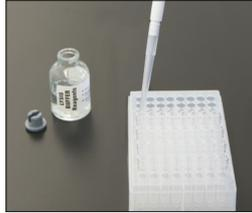
2. Add 450 µL of lysis reagent solution to the sample.
