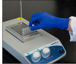
3. Transfer sample tubes to 37°C heat block and incubate for 10 minutes. Then transfer the lysis tubes to the 80°C heat block and incubate for 20 minutes.
