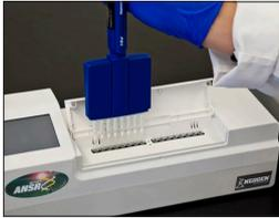
4. Transfer 50 µL of the lysed sample to preheated lyophilized reagents (56°C) in the reader. Cap tubes and vortex briefly. Return tubes to reader. Close the lid and click START in the ANSR software to begin assay.
