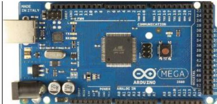
Figura 3.21: Arduino mega 2560
