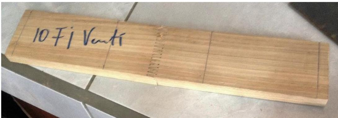
Figura 3.17: Probeta con unión finger joint vertical
