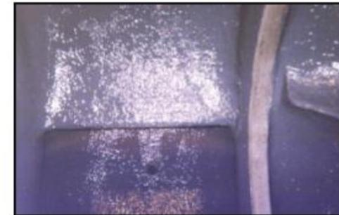
Damaged cutwater rebuilt with ARC 890 and topcoated with ARC 855
