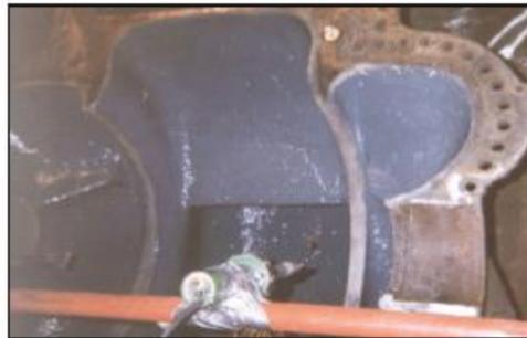
Split case fan pump, coated with ARC 855, ARC 858 and ARC 890
