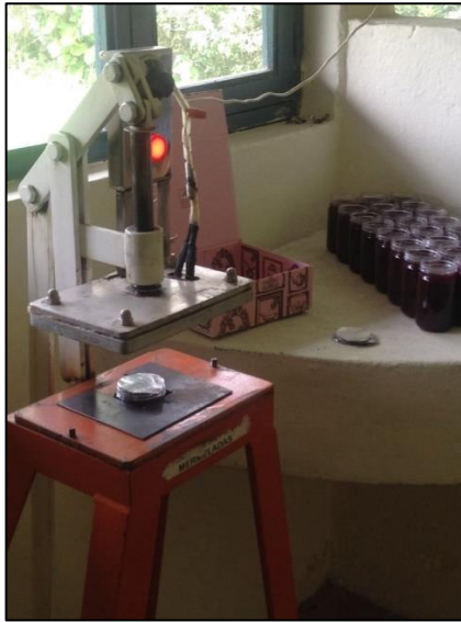
Figure 12: Placing the aluminum shield
